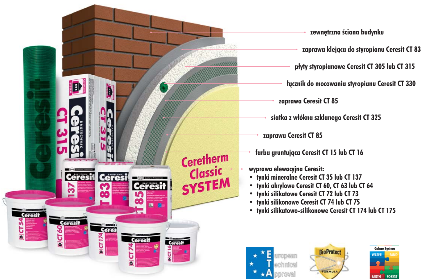
Schemat systemu ociepleń Ceresit Ceretherm Classic.
